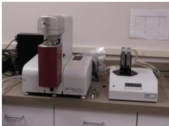
Figure 2: Thermogravimetric Analysis (TGA) used for this report
